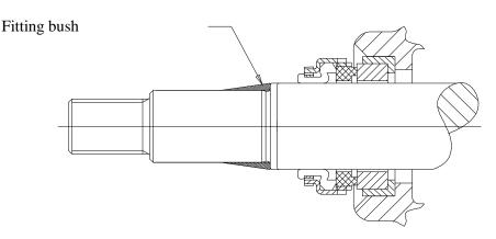
If the carbon ring is not fixed, it is important to check that it is fitted correctly, i.e. the chamfered/lapped side is to face the seat. The carbon ring can be held by a little grease. When using oil on the shaft, the bellows will settle and seat in about 15 minutes, and until then tightness should not be expected. After start, check by viewing the leak hole that there are no leaks.
