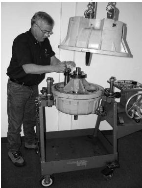
Remove the input shaft.
