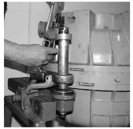
Use a pipe wrench to remove the fitting.
