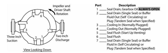
**Note:** Port 5 is the highest point in a vertically mounted pump and should be used for start up venting only.
