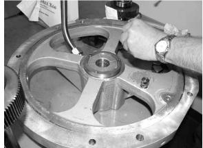
Remove the upper journal bearing and thrust washer, if supplied, from the bearing plate.
