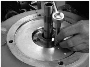
Install upper shaft sleeve and o-ring 936K.
