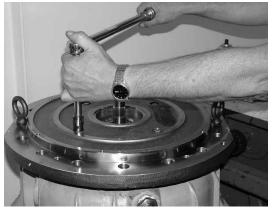
**Note:** Torque seal housing bolts to 35-40 ftlbs.
