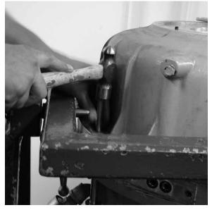
Note: Alignment bolts are close tolerance and must be removed first or damage may occur to the aluminum housing. Damage to the alignment bores can cause increased vibration and reduce gearbox life.
