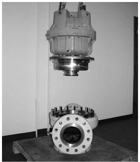
When lifting, if the pump case and seal housing are difficult to separate, use the three jacking screws to break the seal.
