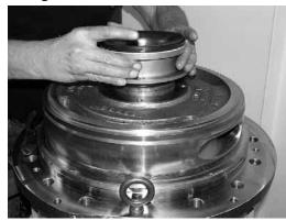
**Note:** Ensure that the inducer tool doesn't rotate while torque is applied on the loading tool.
