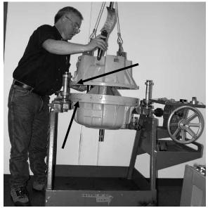
Note: If necessary, a screwdriver (use cloth to protect the aluminum) can be used in the slots to assist in breaking the seal between housings.
