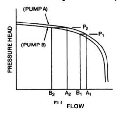
Figure 9. Parallel Operation
