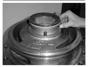
Removing the bolts from the inducer housing.
