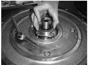
Remove the lower sleeve and o-ring 936J.
