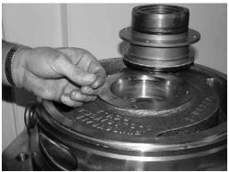
Install the correct shims to maintain the tolerance in the last step. Then install the inducer housing and o-rings 936CA and 936C.
