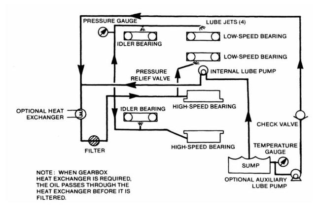
Figure 7. Lube Oil Schematic
