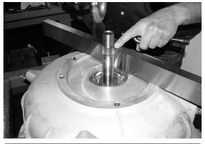
*Note:* Tolerances for shaft shoulder height are 1.203 ± 0.005
