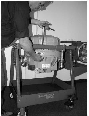
Remove the anti-rotation device.
