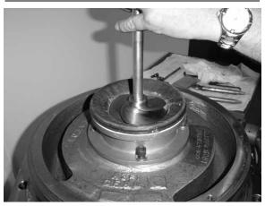
**Note**: When working on a pump with a tapered inducer, the inducer must be removed before the diffuser can be removed from the seal housing.
