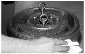
Install the diffuser onto the seal housing.
