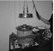
Remove o-ring 936A from the diffuser cover.
