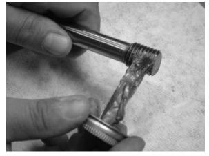
Fully thread inducer stud into inducer loading tool.
