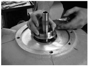
Remove the thermal barrier gasket.
