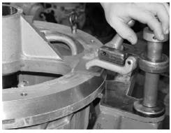
**Note**: "C" clamps can be utilized to perform this task. Be sure to protect the housing faces from any clamping damage.
