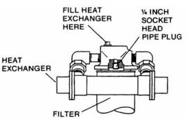
The MA01AA01 Model requires a 1/4" sockethead pipe plug in the filter manifold when using the gearbox heat exchanger. The plug must be removed when the heat exchanger is not being used.
