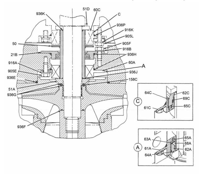
Figure 27. Single Seal Arrangement
