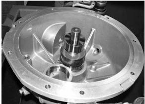
Install upper thrust washer onto the upper journal bearing.
