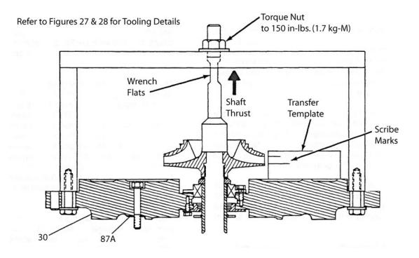
Figure 14. Inducer Housing Adjustment
