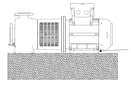
Use shim(s) between motor foot and concrete plinth or base plate to avoid tension in motor foot
