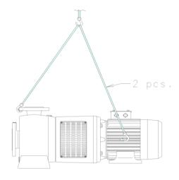
The lifting straps must not bear against sharp edges and corners.
