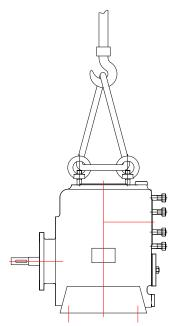
Screw lifting eyes into the pressure flange and mount lifting straps The lifting straps must not bear against sharp edges and corners.
